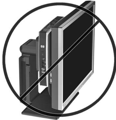
Figure C-9 Unsupported mounting position—thin client between stand and monitor
